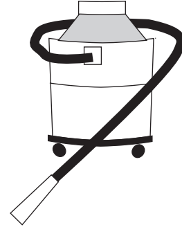
Shop vacuum for cleaning out dust and debris from cracks and spalls
