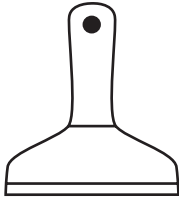
Sharp scraper for shaving off cured material.
